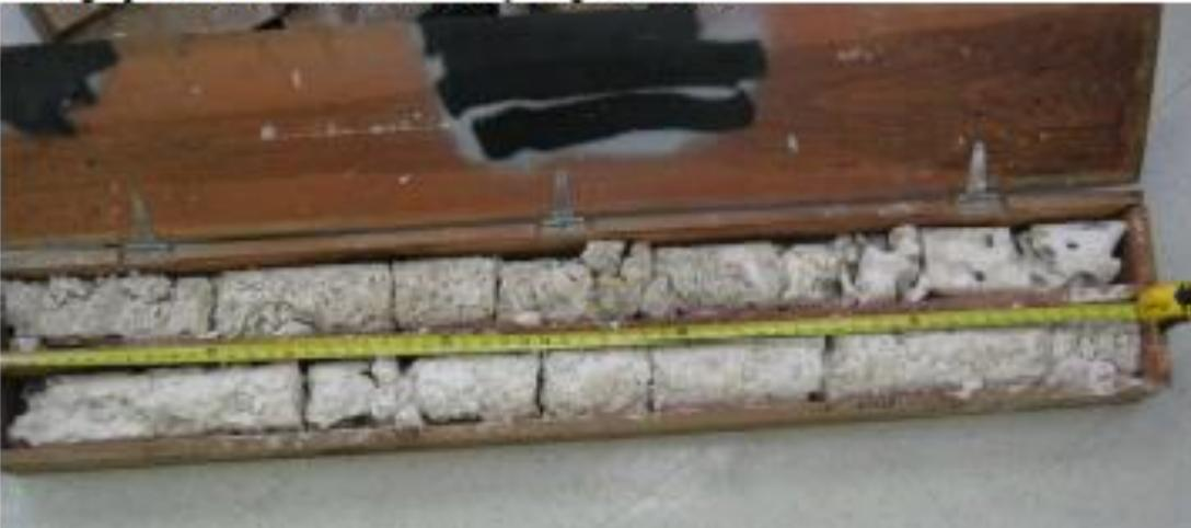
**Photograph 9** – Core box 58 – 68 ft. with close up of hard zone at 62 – 63 ft. Note that the sample was washed to show the burrows that had been filled with soft carbonate.
