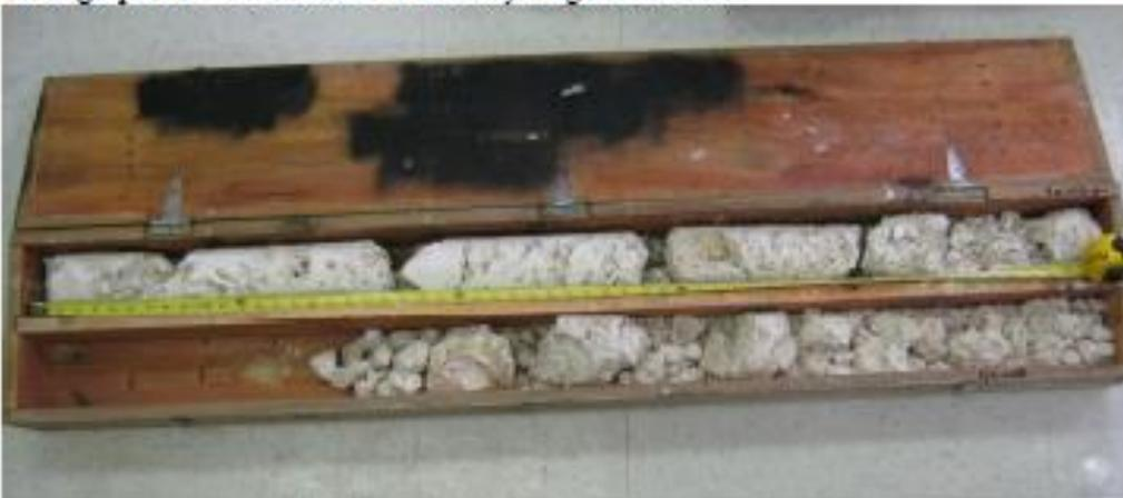
Photograph 15 – Core box 103 – 118 ft. Key Largo Limestone very poor to no recovery.
