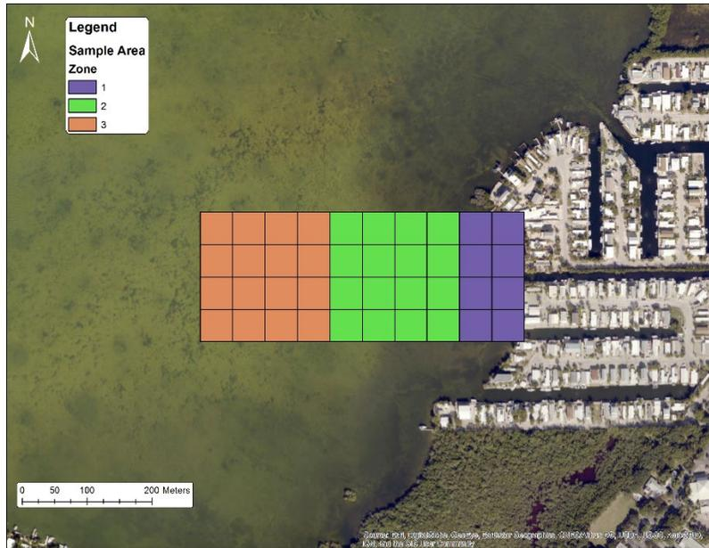
Figure 2: Illustration of the block design to sample water quality from inshore to offshore from canal openings in the Florida Keys. A grid will be established in GIS that will extend 200 meters perpendicular to the mouth of the canal, and 500 meters offshore.
