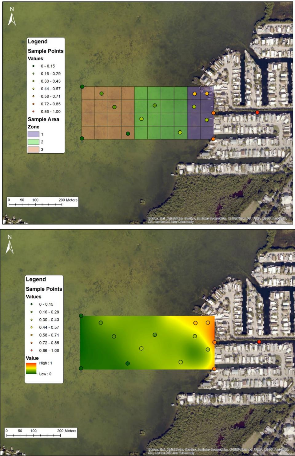
Figure 4: Examples of values for a parameter that has a maximum value of 1 and a minimum value of 0 (Top) and that dataset's corresponding interpolated surface (Bottom).
